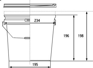
Measurements in millimetres
